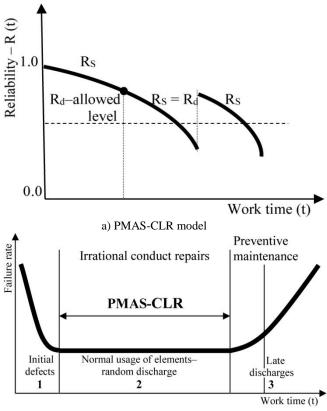
b) Recommendation for maintenance technical systems (TS) Fig. 2. Model of maintenance PMAS-CLR
