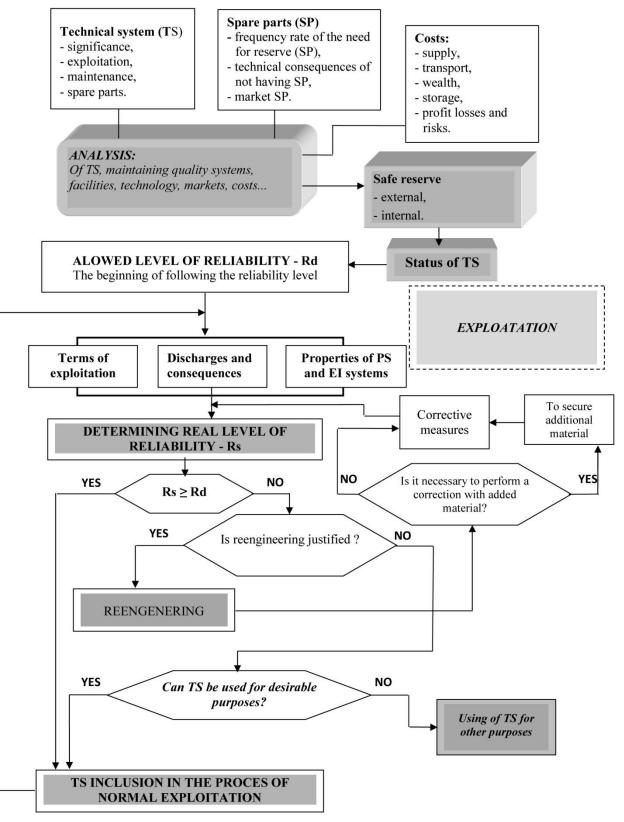
Fig. 3. Flow of control and correction of the reliability level with the safety reserve identification
